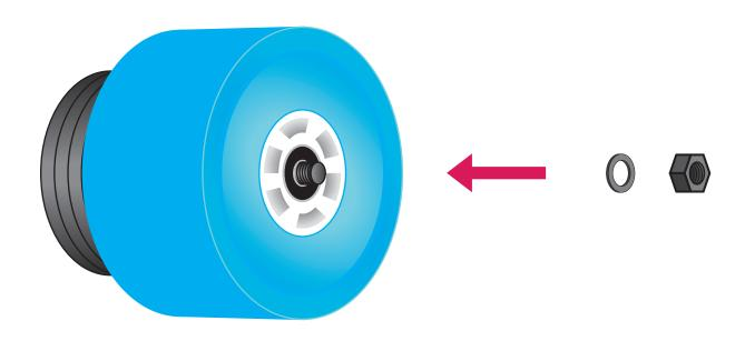
7. Now for the front wheels - they are very easy to remove. Simply unscrew the nut using your T-tool socket. There will be 2 thin washers that you will need to save and reuse on your Street Wheels. One is found just under the nut you removed, and the second is between the wheel and the Truck.
