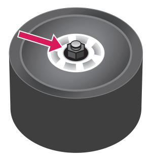
2. With some force, you can pull off the rear motor wheel. If it's proving tough, you can use a rubber mallet and start hitting up on the wheel from underneath, rotating in between each hit. You can put some force into it, the rubber mallet won't damage your wheels.
