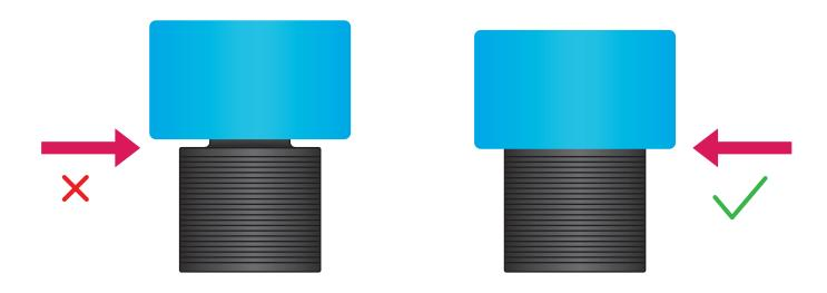
6. Finally, place the washer and the nut onto the shaft, and tighten down. Tighten it all the way down by hand. For best results please do the following: Tighten the nut by hand until you cannot tighten anymore - and then untighten by half a turn (180° counter -clockwise).
