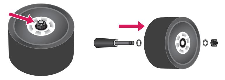
8. Install your Street Wheel - Slide the wheel in the following order - Washer, Wheel, Washer, Nut. Tighten the nut all the way down by hand, then release by half a turn (180° counter-clockwise).
