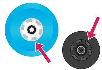
5. Slide the wheel onto the shaft, matching up the prongs to the holes of the wheel. Press down until the wheel sits flush against the motor.
