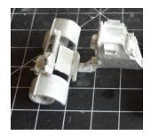
Glue the mud flap as shown and then glue the assembly to the rear axle.
