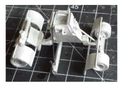
Attach the boom with thread. The boom should not touch the ground.
