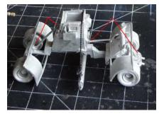
Glue the steering column and gas line as shown.
