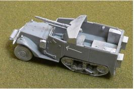
The gun barrel and mount are positioned as shown. The barrel would rest in the windshield groove when traveling and would be elevated above the groove when firing. Attach the gun shield so the shield corners align with second groove in the side.
