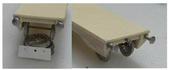
Step 6: The chain is used to connect cars. Glue it on or use separately as you wish.
