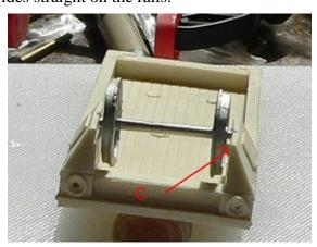
Step 3: Glue the wheels to the axles being sure that they snug right up against the step. If the axles are snug to the step and perpendicular to the flat car body they will be in exact gauge to sit on the track.
