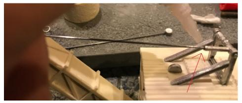
After making sure the alignment is straight and centered (from a side and top view), place a drop of glue on the near crane arm where the wire fits into the arm support.
