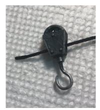
Thread the other end of the thread through the hole in the crane hook. The crazy glued end will pass easily without causing the thread to unravel.
