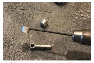
Drill the holes that hold the far end of the crane arm wire supports x2.
