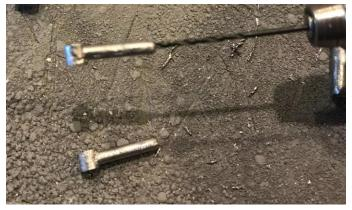
Drill the near end of the crane arm wire supports x2.
