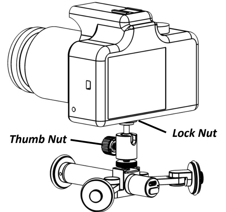
1. Twist the  $\frac{1}{4}$ -20 screw of the ball head into the camera.
