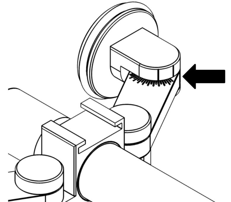
Use the reference lines on the wheel bracket and the swing arms to position the wheels. Some later models have markings on the bottom side of swing arms.
