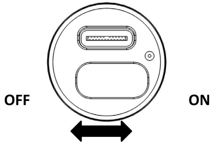
*\*The device turns itself off after 10 minutes of idle. You must reset the device by turning power OFF and ON again to restart.*
