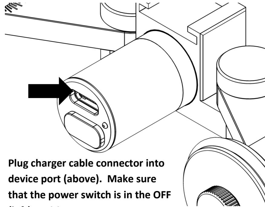
Plug charger cable connector into device port (above). Make sure that the power switch is in the OFF (left) position.
