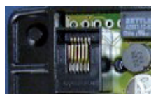
Optional plug-in screw terminal or RJ12 socket
