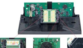
The motion field pattern (wide or narrow) can be changed by rotating the microwave module
