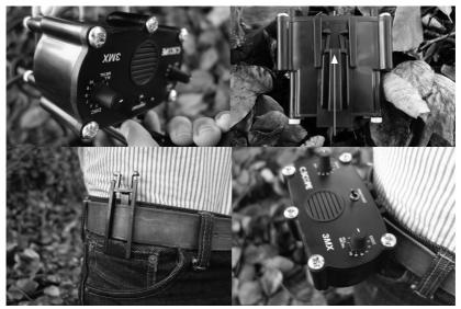
Above: Slide the belt mounting clip into the fixing slots on the underside of the control box and push all the way until the retaining lugs click into position.
