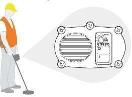
Detection of a metal cover is indicated by an audible pitch increase and target light brightness increase. Small metal targets are ignored.
