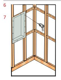
Step 6- Install The Tile Niche into the framing. Push the outside flange onto the front face of the framing. Allow silicone to compress as the flange is pushed against the frame.
