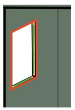
Step 8- Run two beads of Silicone at least 10mm wide all the way around the inside of the framing timber (green).
