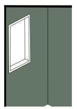
Step 9- Install the Niche into the opening. Ensure the flange of the Niche is pushed onto the wall linings evenly.
