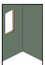
Step 7- Install finished wall linings onto the wall substrate. As above ensure the linings are cut tightly to the Niche opening, and are fixed tightly to the edges of the opening.
