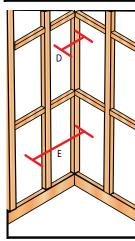
Step 3- Measure from the inside corner of the wall out to the preferred position of where the inner edge of the Niche will be installed (D). Using a level mark this position on the adjacent studs and down to the bottom plate.
