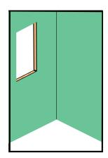
Step 6- Install wall substrate over the framing and fix according to substrate instructions.
