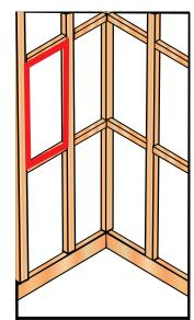
Step 4- Frame out the wall, or modify existing framing so that both sides, and the top and bottom of the niche are surrounded by framing.
