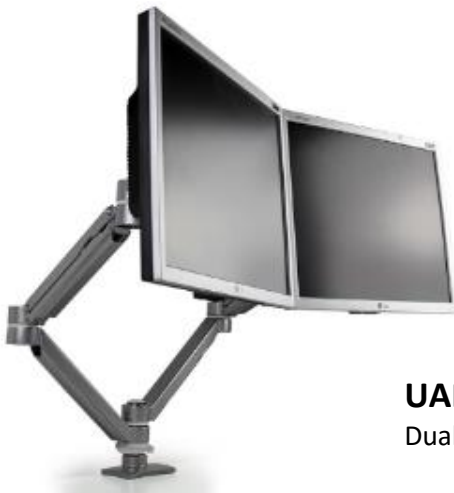
UAMDCR-S Dual Monitor Arm with Cross Bar - Silver Dual screen, double extension cross-bar with one height adjustable segment Counterbalanced spring technology allows for a 2lb to 20lb load
