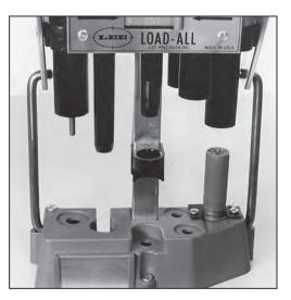
**STATION 5** Immediately move the shell into the shell holder at STATION 5 and complete the crimp. You should have a perfectly crimped shell with a nice, tapered end.
