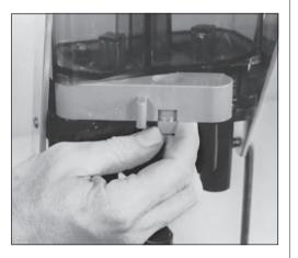
**3** Remove two screws holding the nameplate. Remove charge bar and install correct shot bushing and powder bushing as shown on the charge table. Reassemble, being careful to not overtighten the screws.
