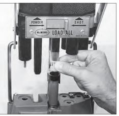
**STATION 3b** Raise handle, insert proper wad and lower the handle until it stops.
