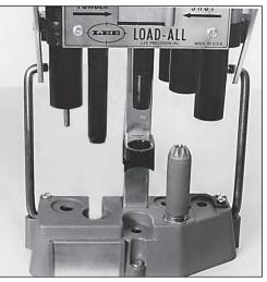
**STATION 4** Place the shell under the proper crimp starter. Keep an inward fold of the shell mouth toward the front for proper alignment with the segmented starter. Depress the handle to a full stop. Some shells may require a two-second pause to set the plastic.
