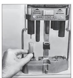
STATION 1 Slip the sizing die, grooved end up, over the shell. Place the shell in STATION 1 and pull down the handle. This will full length size and deprime the shell.
