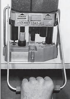
**STATION 2** Place a primer in the priming pocket at STATION 2. Move the shell onto STATION 2: pull down the handle. The sizing die will automatically be pushed off at this station. Remove it completely from the shell.
