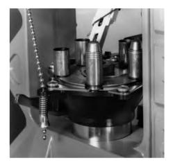
With the carrier in the down position, thread the chain through the outer most hole in the Pro Auto-Disk actuator lever. Raise the ram slightly and pass one full bead through the hole. At this point the chain should be taut between the carrier and the actuator lever. Pass the remaining chain through the inner most hole and pull it tight.
