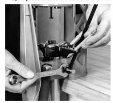
upper most ram travel, place a case in front of the shell slider, cycle lever, again place case in front of slider, cycle lever. If the case collides with the case in shell plate, remove feed rod and unscrew feed bracket one or more full turns. When tightening feed bracket, be sure to allow 5/16" clearance between carrier tongue and square rod—about the thickness of a pencil.
