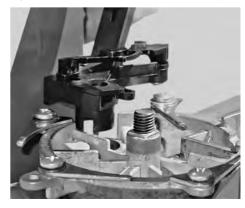
spring is installed into the hole at the rear of the primer punch. Now slip the primer trough over the punch. Push down on the left end of the priming rocker arm to be sure everything is working freely. The primer punch will be seen moving up as you push down on the priming rocker arm.
