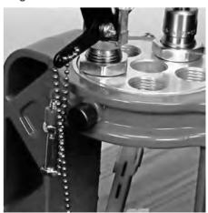
Fine adjustment is easiest done where the chain attaches to the powder measure. The chain passes through two holes in the lever and it will never move, yet it is easily adjusted.
