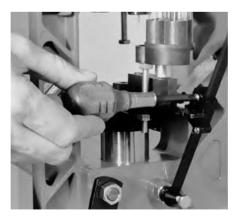
Tighten top screw. Adjust shell insertion pressure with bottom screw.
