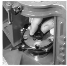
Place case ejector directly on top of the shell plate making sure square on top of center post is engaged and case ejector pointer is towards the chute on the right.
