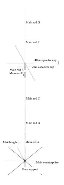
■ VG4 antenna can be adjusted to frequency band center frequency point that we need. During the adjustment, the adjustment of the high frequency band shall affect the low frequency band, while the adjustment of the low frequency band shall not affect the high frequency band. Therefore, the adjustment sequence is: to adjust from 10m of high frequency band to 40m of low frequency band. Generally, only 40m frequency band needs appropriate adjustment.
