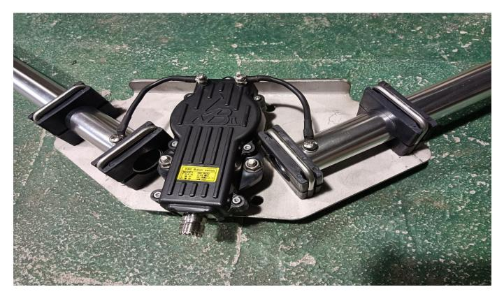
Note: When installing the array mounting bracket, pay attention to the differentiation of the plastic insulating components. The plastic components with steps should be placed at the bottom of the array.
