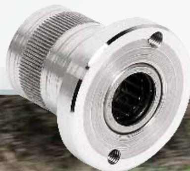
**LEFT:** A new spigot bush with standard MX5 internal bearing is fitted into the end of the MGB crank. Note the two threaded holes which allow bolts to be fitted to push this out if the crank should need replacing or machining in the future.
