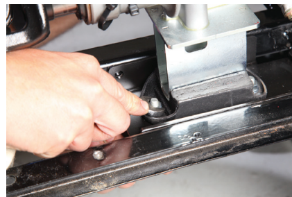
The rear rubber mount is fixed loosely to the bracket. They need to be no more than finger tight at this point as the final position will be determined once the transmission tunnel has been fixed back in place.
