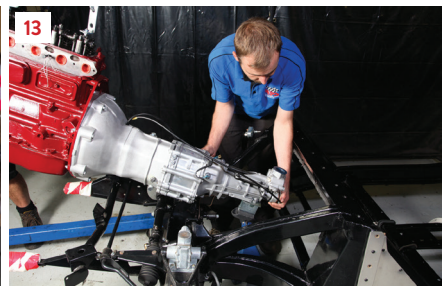
Once the gearbox slides home, fit the top two nuts and bolts to secure in place. Note that the length on the bolts vary around the bell housing.
