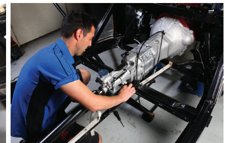
The rear rubber mount is fixed loosely to the bracket. They need to be no more than finger tight at this point as the final position will be determined once the transmission tunnel has been fixed back in place.
