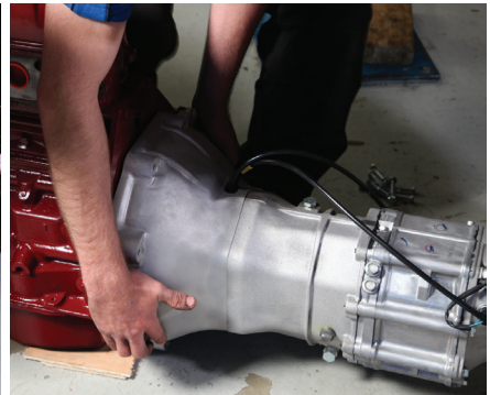
The engine back plate should be cleaned carefully before the box is mated up. There are no dowels to aid location so an extra pair of hands will be very useful at this stage.
