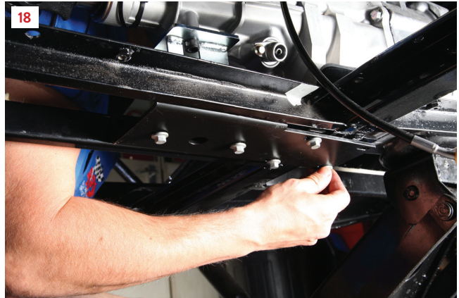
18 The front of the gearbox mount is secured to the cross member using four M8 nuts and bolts. The bottom of the mount should align with the longitudinal members of the chassis.
