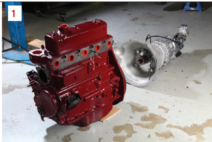
The MX5 gearbox supplied ready to fit, assembled into its custom casing and bell housing, with concentric slave cylinder ready fitted. It's even already filled with the correct gearbox oil.
