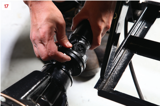
17 ... and the propshaft rear flange is bolted up to the differential.
