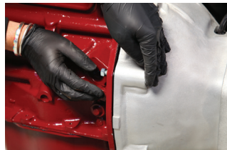
Once the gearbox slides home, fit the top two nuts and bolts to secure in place. Note that the length on the bolts vary around the bell housing.
