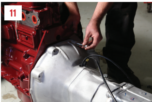
Once the gearbox slides home, fit the top two nuts and bolts to secure in place. Note that the length on the bolts vary around the bell housing.
