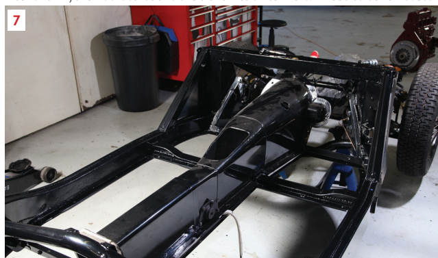
If you're working on a complete MGA, you will need to remove the propshaft before removing the transmission tunnel.
