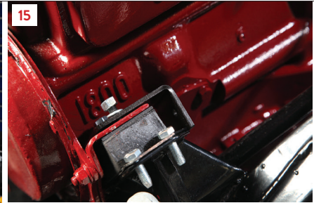
15 On the left-hand mount, the engine restrictor bracket is fitted. This prevents the engine moving forward should the mounts fail for any reason.
