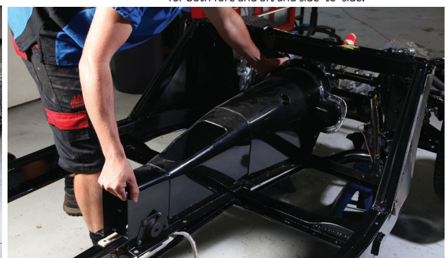
If you're working on a complete MGA, you will need to remove the propshaft before removing the transmission tunnel.
