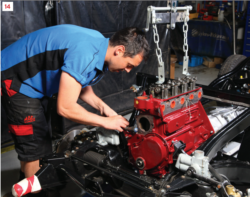
14 With the gearbox supported on a trolley jack, the engine mounts are aligned and the fixing bolts slotted into place.
