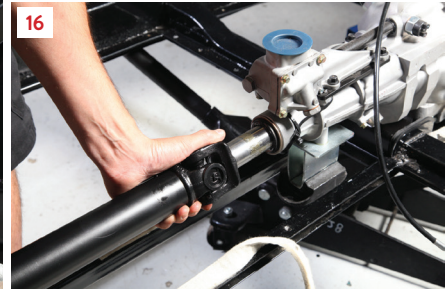
16 The propshaft yoke is lubricated with some gearbox oil and then slid into the gearbox...
