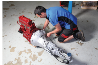
Once the gearbox slides home, fit the top two nuts and bolts to secure in place. Note that the length on the bolts vary around the bell housing.
