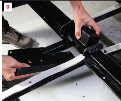
The new gearbox mount is secured by four nuts and bolts. It fits snugly between the longitudinal rails which require two holes drilling on each side.
