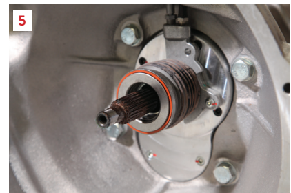
The concentric slave cylinder comes pre-fitted with all necessary pipework – a banjo ended pipe which goes to the master cylinder and a bleed pipe. These exit through the top of the bell housing and need to be handled with respect during the fitting process.
