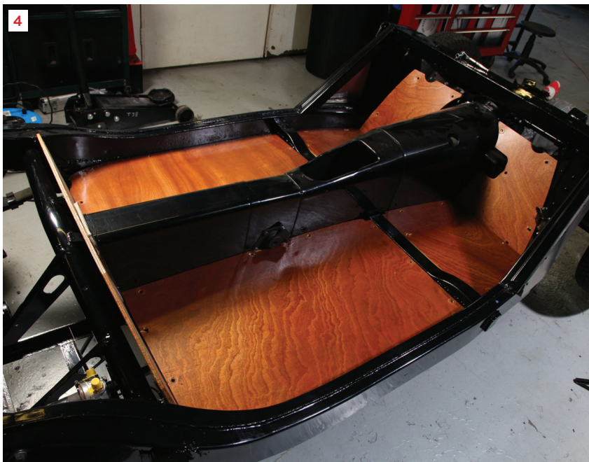
As we're fitting the gearbox into an effectively bare chassis, we can pre-assemble the engine and box as a unit and fit from the front. If you're going to fit just the gearbox, it's necessary to go in through the car, meaning all interior trim, the floorboards and the transmission tunnel will need to be removed.
