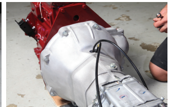
Once the gearbox slides home, fit the top two nuts and bolts to secure in place. Note that the length on the bolts vary around the bell housing.
