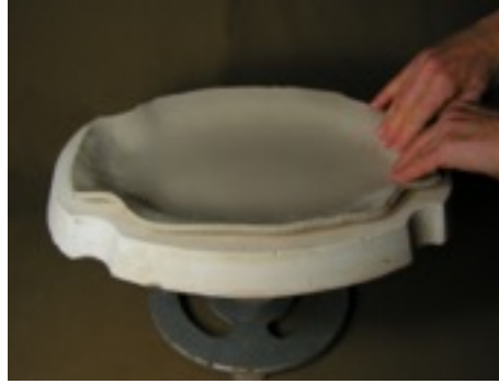
Ease Slab into Mold
