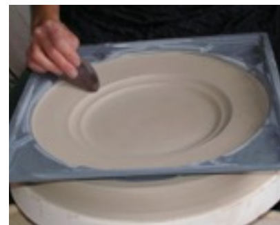
Insert slab and then shape
