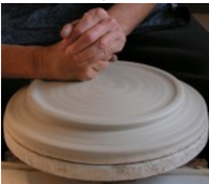
Draw clay down and shape foot.
