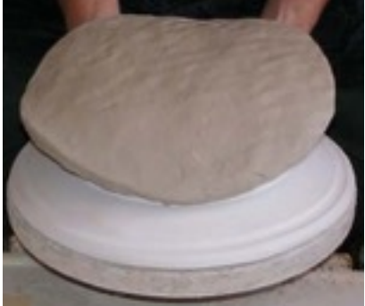
Apply clay paddy to bat. Press straight down with side of your fist to adhere.
