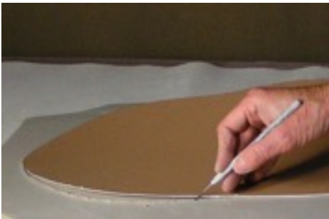
Cut slab around template
