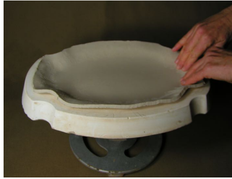
Ease Slab into Mold
