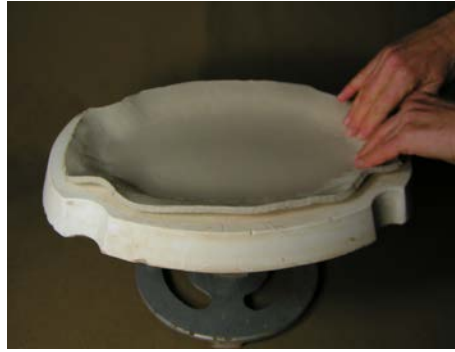
Ease Slab into Mold
