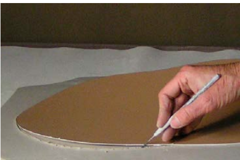
Cut slab around template
