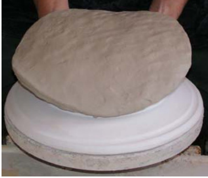
Apply clay paddy to bat. Press straight down with side of your fist to adhere.
