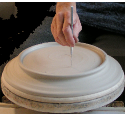
Test for even thickness. Then compress plate with a wooden rib.
