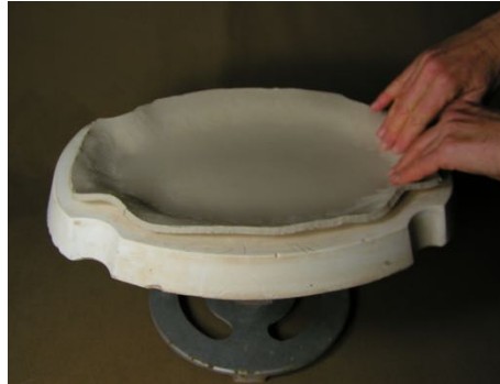
Ease Slab into Mold
