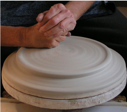
Draw clay down and shape foot.
