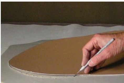
Cut slab around template
