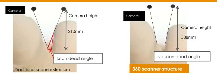
From the analysis of scanning principle from binocular vision imaging, the gap is blocked easily when the camera is closer to model being scanned, the larger the scan dead angle is: Conversely, smaller.
