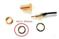
The split washer should not be used on thick plastic enclosures (use it only on thin metal enclosures). Ensure the aerial cable is fully screwed together – the threaded end piece will become loose during shipping!
