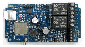
The Network Fault LED lights when there is a problem with the network service. This is normally due to the SIM not having sufficient credit.
