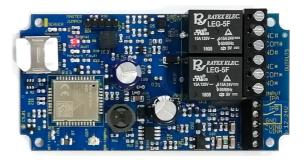
The No Signal LED lights when no GSM signal can be found Check the aerial is fitted correctly. The LED will flash when the signal strength is less than 11. Keep the aerial away from wires and metallic surfaces
