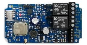
The SIM Fault LED lights if the device cannot use the SIM Check the orientation of the SIM and remove all PIN numbers or set them to 0000
