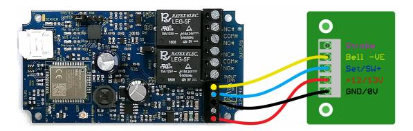
When first powered up, the flashing network LED will initially flash at a rate of once per second. This will slow to once every 2 seconds once a network connection has been established. If the device cannot acquire a connection a fault light will illuminate to indicate the cause of the problem.
