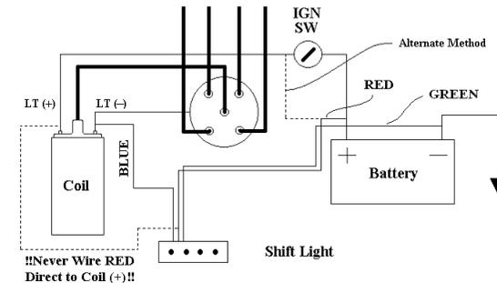
Figure 1. Conventional Ignition Wiring Diagram
