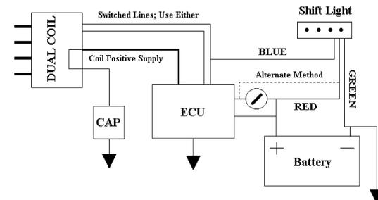
Figure 2. Wasted Spark Distributor-less Ignition Wiring Diagram
