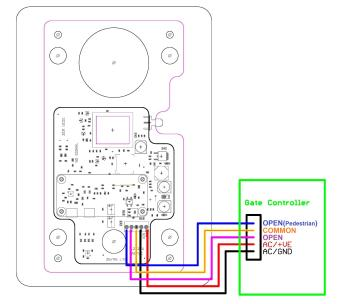
The absolute maximum supply voltage is 24V AC or DC. The VIN terminals are not polarity sensitive and can be connected either way around. Current consumption varies from 25mA at idle to 200mA when active.
