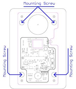
Using the supplied stencil, drill the four mounting holes and the cable entry hole onto a flat surface. The maximum size for each hole is marked on the stencil.
