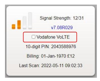
Ensure the Vodafone VoLTE checkbox is ticked when using Vodafone 4G
