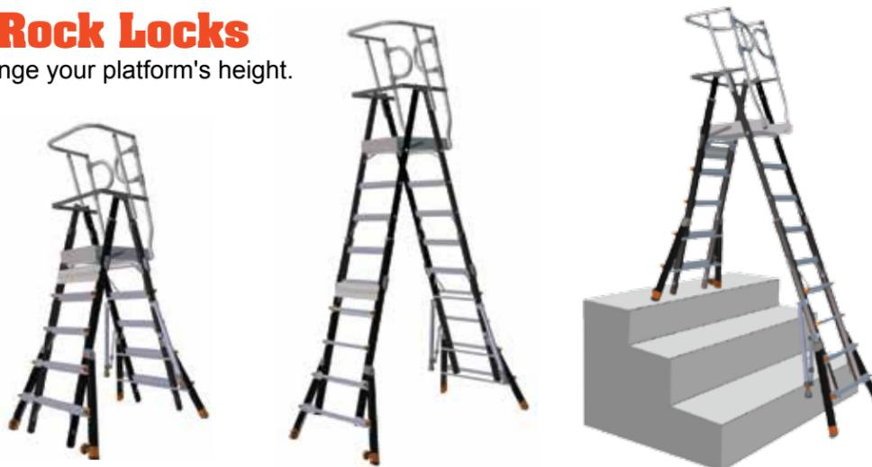
The Rock Locks adjust the height of the Cage. Push in on the bottom of the Rock Lock to open, tap the Rock Lock to close. Unlock only one Rock Lock at a time while supporting the inner ladder assembly with one hand. Do not unlock the Rock Lock if anyone is on the Cage.
