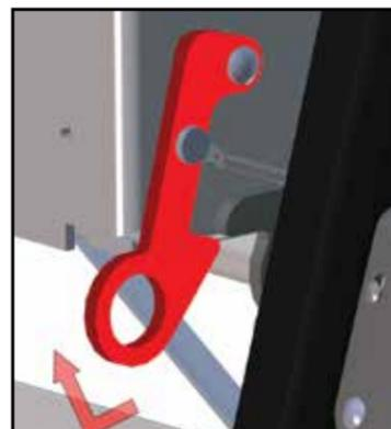
Lower the cage height to the shortest position, pull the locks out and up to release the platform
