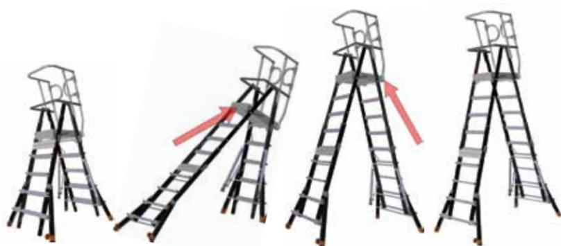
Begin from the small A-frame position. Stand to one side of the Cage; unlock both Rock Locks on one outer section. (When extending the Cage your hands must always be on the outside of the outer section). Place one hand on the Platform or upper inner rails and push the inner section away from you to extend the Cage. Once you have reached the desired height, line up the inner and outer rungs, then lock both Rock Locks.
