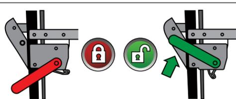
Lift up on the rope brake to carefully lower the inner section down.
