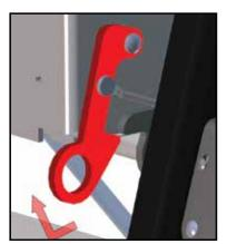
Lower the cage height to the shortest position, pull the locks out and up to release the platform
