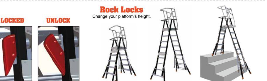
The Rock Locks adjust the height of the Cage. Push in on the bottom of the Rock Lock to open, tap the Rock Lock to close. Unlock only one Rock Lock at a time while supporting the inner ladder assembly with one hand. Do not unlock the Rock Lock if anyone is on the Cage.
