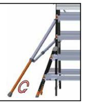
Extend leg down until firmly seated Twist counter clock-wise to lock
