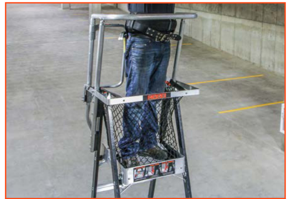
Enclosed work platform
