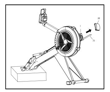
2. Position the Main rd Hook(12L) from the Main Frame(1). Make a mark on the Bungee Cord (38) to move the hook forward 2 inches. Refer to View 1 to View 3 to untie the Bungee Cord (38) from the Left Bungee Cord Hook(12L), and move the hook forward 2 inches. Refer to View 4 to View 6 to retie the Bungee Cord(38) to the Left Bungee Cord Hook(12L). Hook the Left Bungee Cord Hook(12L) back into the Main Frame(1) and push the hook to the left side to touch the inner wall of the Main Frame(1).
