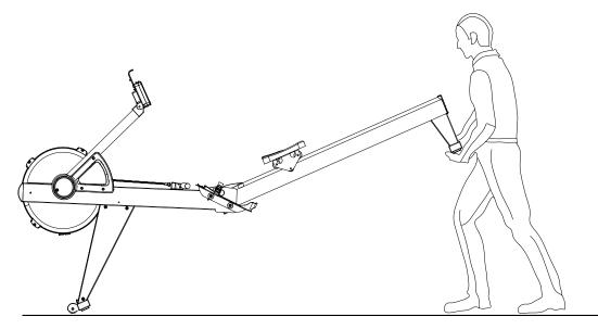
4. The Main Frame(1) and the Rail Frame(2) can be separated to minimize the unit size for storage. Remove the Pull Pin(98) from the Main Frame(1). Lift up the Main Frame(1) and pull out the Rail Frame(2) to separate. Insert the Pull Pin(98) back to the hole in the Main Frame(1) for storage.
