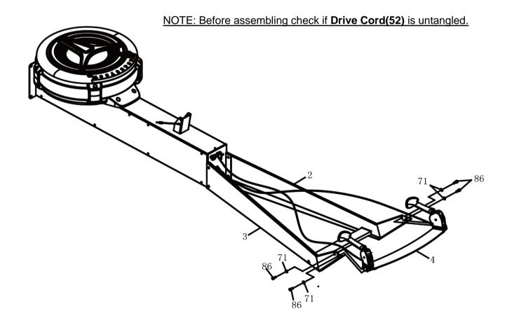
Make the assembly stand up. Tighten the Left and Right Upper Arms (2/3) using: 2 PCs of M8x12mm Socket Head Cap Screw (86) and M8 Flat Washer (71). Then tighten all bolts.
