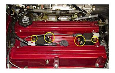
**Step 2:** Insert the new JDC ignition system and plug in the connectors to the factory harness on both sides. They will snap into place when fully inserted. Press firmly on the top of each coil to make sure the coils mount flush to the valve cover.
