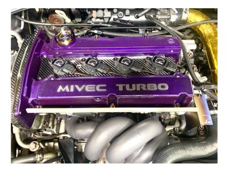
**Step 4:** Hold the heat shield down on the valve cover as you tighten the bolts. (Occasionally the threads on the bolts will grab the heat shield and start to pull it up. If this happens, push the heat shield back flush to the mounting hole before proceeding to tighten the bolts.)
