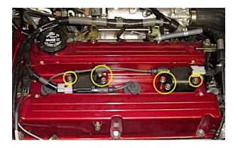
**Step 2:** Insert the new JDC ignition system into the valve cover and press firmly on the top of each coil to make sure the coils make contact with the spark plugs. They will not snap into place, but you should feel the rubber boots slide over the spark plugs.
