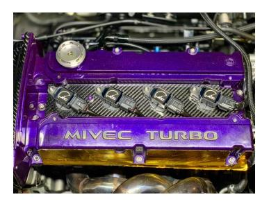
**Step 3:** Use the included hex head bolts with washers to secure the mounting plate to the valve cover and tighten. The wire harness will need about 1/8" for the wires to come through on the right side. Make sure to use the attached washer as a spacer on the right side to leave room for the wire harness to come out under the plate without being pinched. Be careful not to tighten too much. This may result in stripping the threads on the valve cover or pinching the wires.
