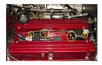
Step 2: Insert the new ignition system into the valve cover and press firmly on the top of each coil to make sure the coils make contact with the spark plugs. They will not snap into place, but you should feel the rubber boots slide onto the spark plugs.
