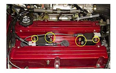
**Step 2:** Insert the new JDC ignition system and plug in the connectors to the factory harness on both sides. Press firmly on the top of each coil to make sure the plate mounts flush with the valve cover.
