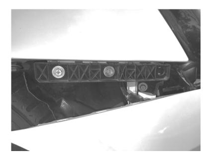
**Step 3:** Remove the 10mm bolts that hold the brace in place and pinch the black tabs from behind to remove the brace.
