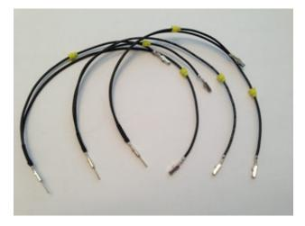
**8.** Crimp Denso pins to the end of each wire. There should be 12 total including both sets of wires. <u>Do</u> <u>not</u> plug them into the connectors yet.
