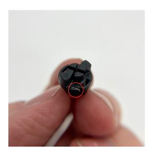
5. Using your pick or tweezers, push the wire out of the slot and pull it up straight. Turn it around to the other side and repeat for the other wire. Your bulb should now look like the one in the picture below.
