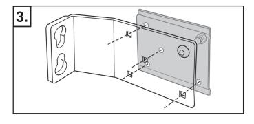
**Important:** To ensure the fit of the backing plates the 3/8" mounting bolt holes must be drilled acurately, perpendicular and straight through the door.
