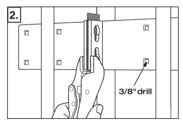
Place a thin strip of card stock between the hasp sides to prevent binding after installation. Check their alignment and clamp them together with the vice grips.
