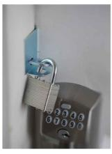
4. Secure with a padlock or security seal. Add the optional lockout tag with contact information.
