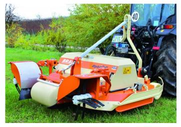
Vine Trunk Cleaner *RP W 1* (single rotating shaft) attached to Mulcher/Mower *Alpha sensotronic*
