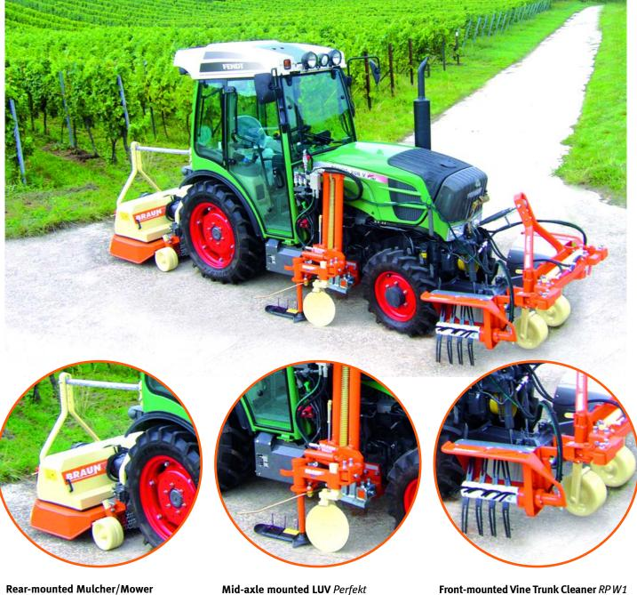
For mulching the vine trunk wood in spring or controlling grass throughout the year. Combining several BRAUN implements and attachments ensures your work is efficient and environmentally friendly. Soil compaction is reduced as a result of fewer tractor passes.
