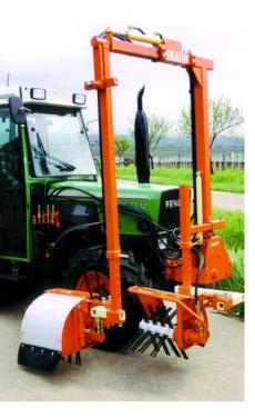
Vine Trunk Cleaner *RP W 1* (single rotating shaft) frontmounted with over-row frame With the over-row frame you can cultivate terraced terrain by adjusting the inner wheel cylinder. This way you only need to keep your eye on one row at a time.
