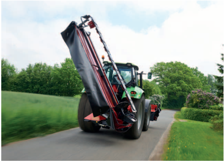
Up to 125° vertical transport position for excellent weight distribution.
