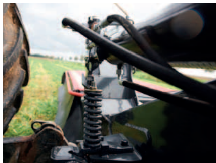
When encountering an obstacle the NonStop BreakBack system protects the cutterbar by swinging it back and up.
