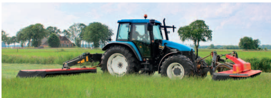
Centre mounted suspension for even weight distribution and fast adaptation to ground contours.
