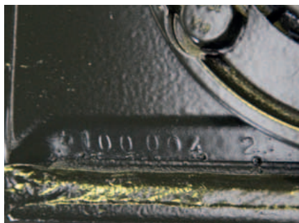
Every cutterbar is given a unique number, making it easily identifiable for future reference.
