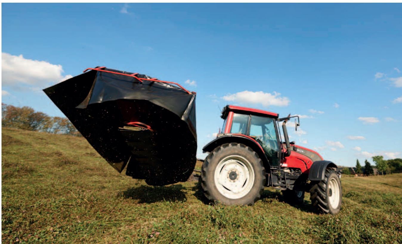
Lifting on headlands via a hydraulic cylinder.
