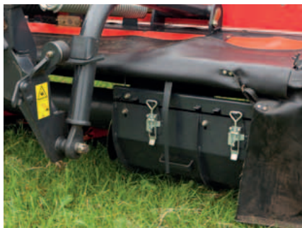
Swath width is easily changed by simply unlocking the swath plates and sliding them to the requested position.
