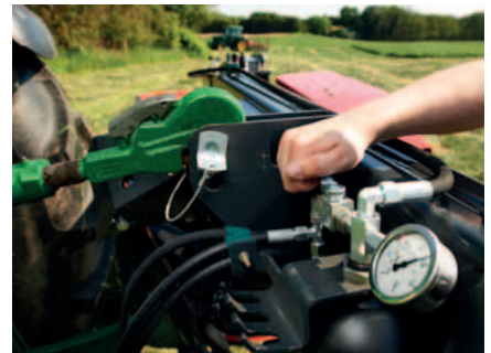
Hydraulic setting of ground pressure (EXTRA 432H).
