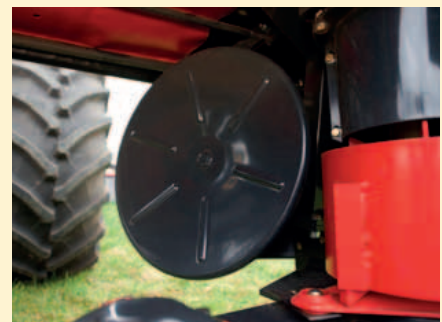
The machine is standard equipped with two swath discs, allowing a swath width of 2.2-2.4 m.
