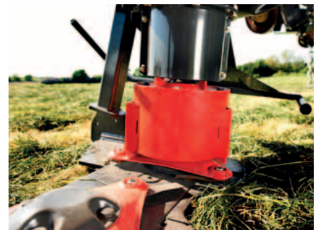
Direct drive from the gearbox to the first disc for efficient power transmission.
