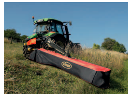
The machine can be operated at an upwards or downwards angle of 15°.
