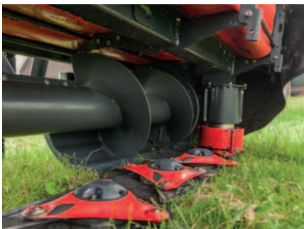
Actively driven swath former, producing even, box-shaped swaths.
