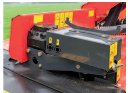
The auger is driven by a small gearbox with an additional power requirement of only 5hp.
