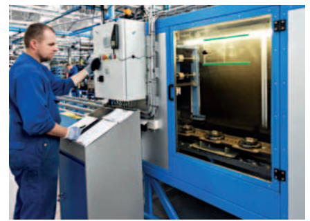
All cutterbars are testrun and checked for noise and heat level.
