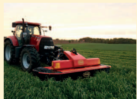
By switching driveline pulleys changing from standard PTO speed of 1000 rpm to 750 rpm is possible.
