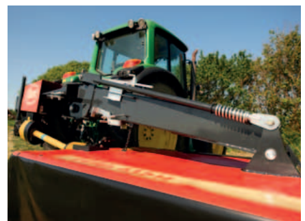
Any ground-unevenness are absorbed by the suspension.
