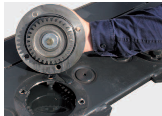
Each individual disc bearing housing can be removed very quickly for easy maintenance and bearing replacement.
