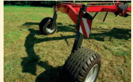
Active wheel steering for improved manoeuvrability in combination with large wheels for reduced compaction.
