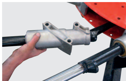
Each tine arm can be dismantled and repaired individually.
