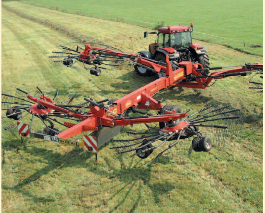
The 2-pt headstock allows a turning angle up to 80°.
