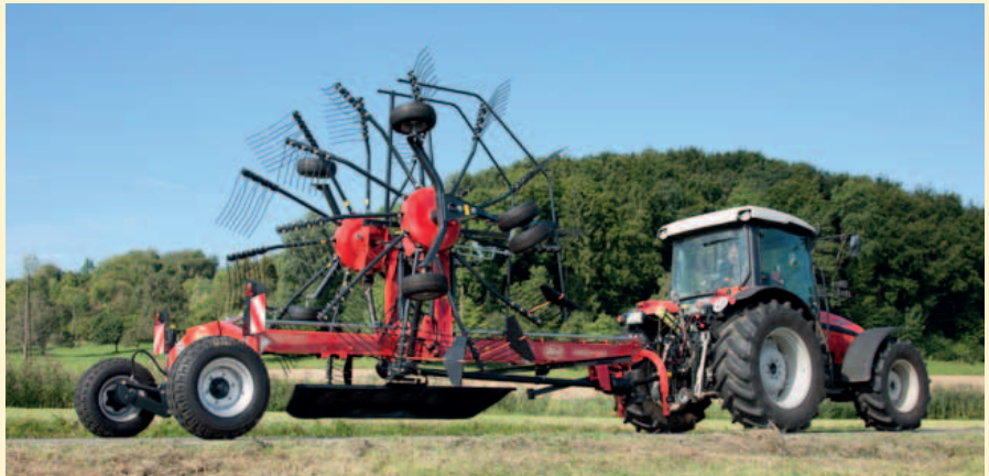
All main functions, such as lifting and lowering of mainframe and rotors are operated from the tractor cab, using an electro hydraulic control terminal.
