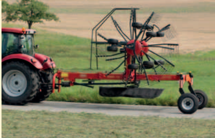
Vicon centre swath rakes are converted hydraulically for transport from the tractor cab.
