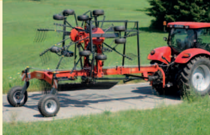
To limit transport height further the tine arms can be removed on the Andex 764. The swath board is folding up automatically.
