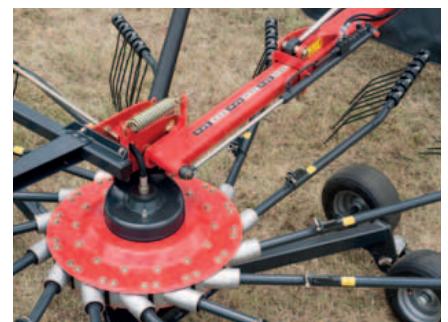
Hydraulic adjustment of working width.
