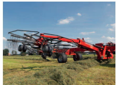
High lift of rotors ensures generous clearance during headlands turns. Clearance height can be adjusted infinitely.
