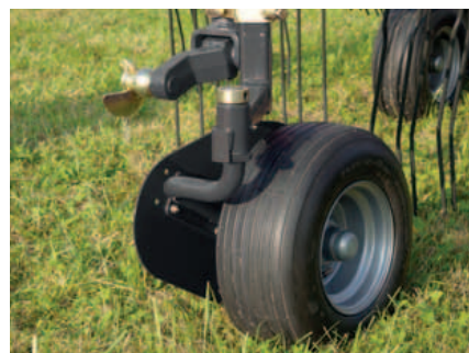
As an option these rakes can be supplied with a third wheel, to ensure even better flotation.
