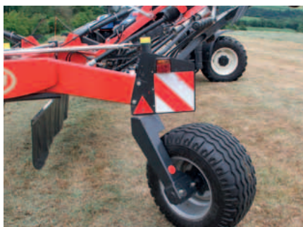
Standard running wheels of Andex 804 is extra wide 380/55 flotation tyres for excellent ground protection.
