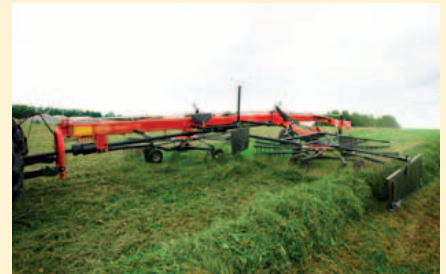
The side delivery concept allows you to collect crop from 15.00m into a single swath.
