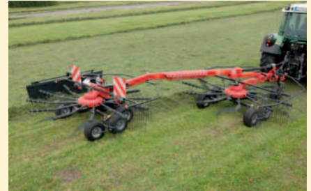
The 714T VARIO with 7.10m working width and unique new SideShift device.
