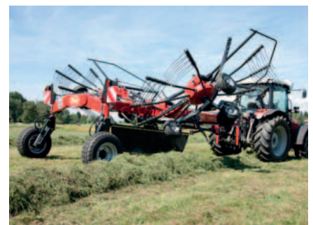
A spring ensures parallel lowering and lifting of the rotors and prevents tines from digging into the ground during headland operation.
