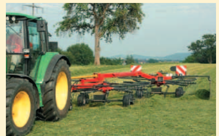
SideShift to the left - raking without driving on unranked crop.
