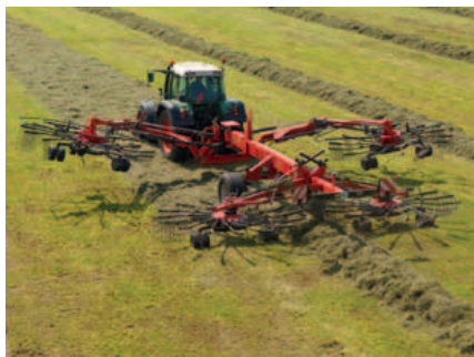
Front and rear rotors can be lifted with adjustable time delay between front and rear, pairwise or individual.
