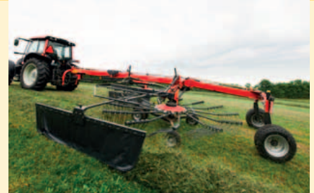
The low position of the rear frame, moves the gravity point close to the ground for excellent stability.
