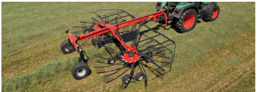
Andex 844 with 8.40m working width, fully enclosed gearbox and hydraulic adjustable working width.
