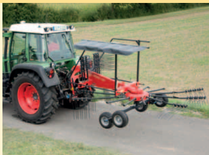
All rakes can be set for reduced transport and storage width by removing the tine arms and placing them on the carrier frame.
