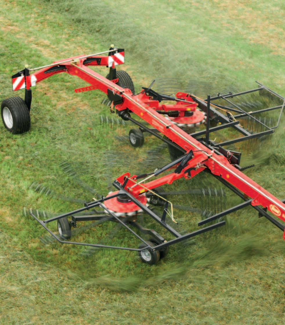
The low position of the rear frame, moves the gravity point close to the ground for excellent stability.
