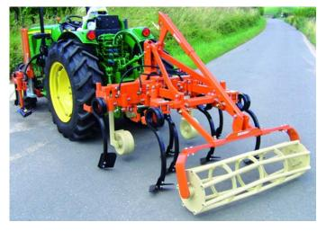
Cultivator *Vario* (Spring tine cultivator) with spring tines, stabilising wheels and pipe roller with three point mounting bracket for depth control
