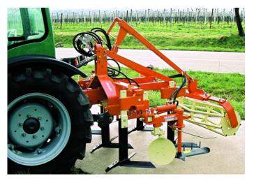
**Cultivator** *Vario* **with five wing tines with shearbolts, LUV** *Perfekt*, **attachable frame and three point mounting bracket for tube roller** For year-round level ground weed control.
