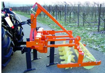
**Cultivator** *Vario* **with five solid tines, chisel feet followed by the spade roller harrow and crumbler roller for depth control** Ideal for slopes because the ground is cut open with the chisel feet and the spade roller breaks up large chunks of soil at a greater depth.
