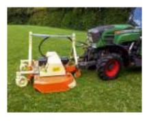
Front-mounted variants for tractors with reversible seat or front attachment for tractors with front power take-off.
