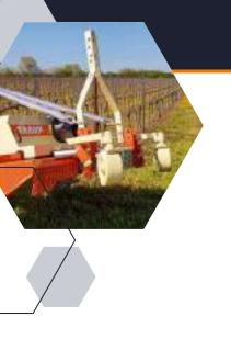
We have integrated mounting brackets to attach additional BRAUN under-vine cultivation equipment. This allows you to expand the mowers of the Alpha series modularly and thus enables you to complete several operations in one.
