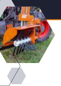
The BRAUN vine trunk cleaner RP W1 and RP W2 is the optimal tool for removing water shoots and for mowing in the under-vine area. Due to the geometry of the rubber punchers and the material composition, the device is particularly gentle on the vines and has a long service life.
