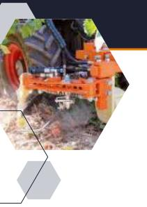
The BRAUN under-vine cultivator is suitable for ploughing off soil masses in the under-vine area. This device has no problem pulling dams and larger masses of soil between the vines into the alley.
