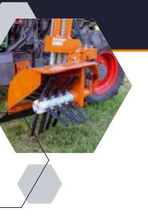
You can attach the BRAUN vine trunk cleaners in the mid-axle area, to BRAUN mowers and to the Vario and UKR implement carriers. This allows you to complete various tasks in one pass.
