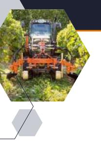
The BRAUN Universal Cultivator Frame UKR is a lightweight implement carrier for mounting on the front or rear hydraulics. The implement carrier has a hydraulic width adjustment for individual adaptation to your row widths. The UKR is characterized by its lightweight design and high diversity of variants. It consists of the UKR base frame, sliding parts and the hydraulic width adjustment.
