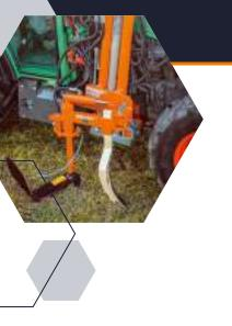
The BRAUN dished ploughshare and cultivator LUV Perfekt is designed for fast and environmentally friendly work around the vine. The flat blade drives under the vegetation between the vines and cuts through the roots of the weeds a few centimeters below the surface. The attachment of preliminary tools such as the concave coulter disc, straight coulter disc and rigid leg with various blades is designed for ease of use.
