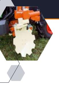
The BRAUN disc plough is a cost-effective device for mechanical weed control in the under vine area. During rotation, the toothed hollow disc cleanly cuts the grass edge, throwing the soil between the vines. Thus, the unloved weeds are covered with soil and disturbed in their growth. In addition, by mounding the soil on the vine, you protect it well from the winter weather. High driving speeds are possible with the BRAUN disc plough.
