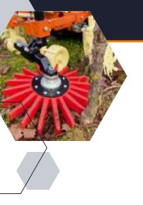
The finger weeder removes weeds directly on the plant very gently and at the same time it levels the soil in the under-vine area. In combination with the rotary star tiller, it is a popular piece of equipment for ecological weed control in the under-vine area. It is available in two different sizes and degrees of hardness.
