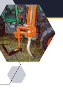
Various root separating devices can be attached to the ploughshares, which separate the roots from the soil after driving under the turf. We also offer extension wings for demounding and demounding knives for pulling out the soil between the vines. Extended by the rotary tiller, the LUV is optimally equipped for actively destroying the root system of the weeds.
