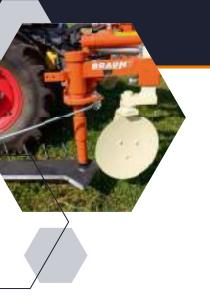
Equip the modular LUV with a wide variety of under-vine implements that - like the standard flat blade – work between the vines and avoid the plants via a hydraulic feeler arm control to prevent damage to the vines. The implements simply attach onto the splined shaft of the base unit.
