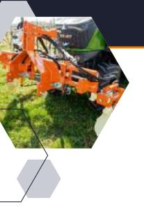
Brackets for the Vario and Vario II implement carriers to hold undervine cultivation implements. such as the BRAUN LUV Perfekt dished ploughshare and cultivator. the BRAUN rotary star tiller. finger weeder and many more.
