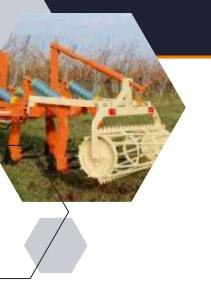
The BRAUN Acticult cultivator is particularly suitable for working in heavy and stony soils. The spring packs mix the soil very effectively.
