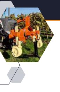
Equipped with the appropriate legs and chisels, the BRAUN Vario or Vario II easily loosen the soil in the alley, mix the upper, humus-rich layer and loosen weeds including roots. Whether as a cultivator in front of cardan shaft driven machines for upstream loosening of hard soil structures, or as a full-fledged cultivator with a second tool level, with BRAUN cultivator tools you will achieve excellent working results.
