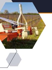
By mowing the greened vineyard areas, you return important nutrients to the soil for humus formation. Our mowers are also ideal for shredding vineyards and sawn timber. The Alpha series is hydraulically adjustable in width and thus suitable for different vineyard dimensions. The BRAUN Alpha series also includes the Alpha sensotronic, which adjusts to the row width independently of the side via the sensors. Manual control of the side sections is also possible via the hydraulic width adjustment.
