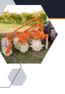
With the help of the BRAUN disc harrow you loosen the upper soil layer, break up clods of soil and thus achieve a good crumbling for seedbed preparation. It also enables a high working speed for weed control. The BRAUN disc harrow packages can be mounted in two rows on the Vario cultivator. The disc angle can be easily adjusted using the hole pattern plate. This means that plowing in and out can be carried out without much effort and without having to change the bolts.
