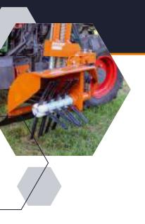
With the over-row frame in the front attachment, you can guide the vine trunk cleaners on both sides of the vine and remove both water shoots on the vine trunk and weeds in the under-vine area much more efficiently. The width and height of the over-row frame can be adjusted hydraulically.
