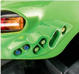
The rear controls on the ProfiLine versions can include controls for an additional remote valve to order.
