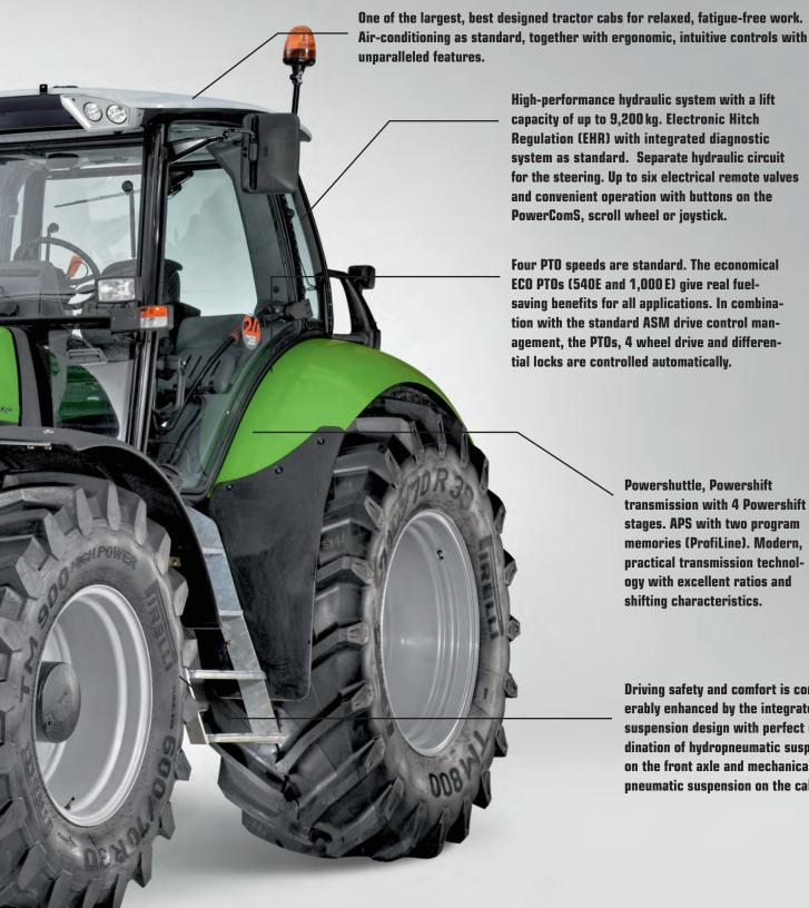
High-performance hydraulic system with a lift capacity of up to 9,200 kg. Electronic Hitch Regulation (EHR) with integrated diagnostic system as standard. Separate hydraulic circuit for the steering. Up to six electrical remote valves and convenient operation with buttons on the PowerComS, scroll wheel or joystick.
