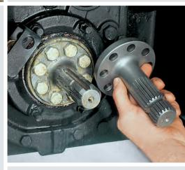
Fast replacement: The screw-connection PTO stub.
