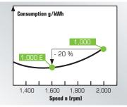
With the economy PTO the Agrotron runs in the optimum consumption range of 1,600 rpm. The speed is lowered by 20% and the consumption by around 12%.
