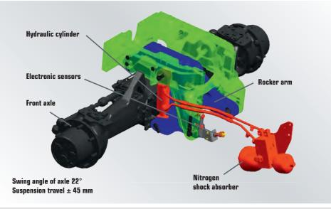
Comfortable and safe: The Agrotron M has hydro-pneumatic front axle suspension.
