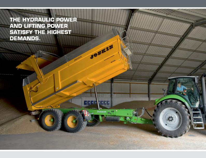
You can never have enough hydraulic power. With this in mind the Agrotron M is fitted as standard with closed center loading sensing hydraulic system which satisfies the very highest demands with a delivery rate of 120 l/min and a system pressure of 200 bar.
