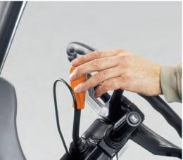
Changing the direction of travel without actuating the clutch: the standard Powershuttle .
