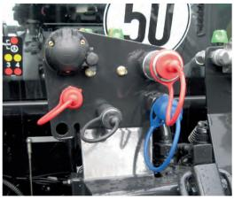
To order the Agrotron M can be fitted with Power-Beyond connectors for the direct connection of third-party devices.
