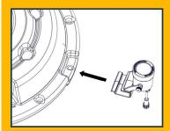
Snap-on light clips are included with each light kit to make installation even easier.
